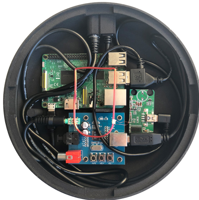
Figure 39. Technical components of Melo : A Raspberry Pi 3, RFID reader and sound card.
